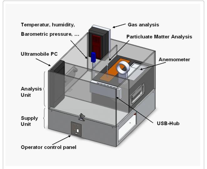
**Figure 1 MAQS-vehicle sensing modules.** Varible positions of sensors with regard to positions within the vehicle (front or back seats) and sensor position height (adults or children height).
