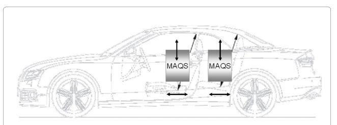
**Figure 2 Schematic illustration of MAQS sensing module**. The module consists of a supply unit and an analysis unit. In the analysis unit, particulate matter analyzer, gas analyzer (i.e. CO2, NO2, CO) and temperature, humidity, anemometer sensors are placed. An ultramobile PC unit integrates the data.
